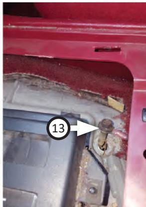
25. Extend momentary switch black ground wire with **splice connector (14)**, **black wire (6)** and **eyelet (13)**. Ground this wire to chassis (this kit was grounded at shifter).
