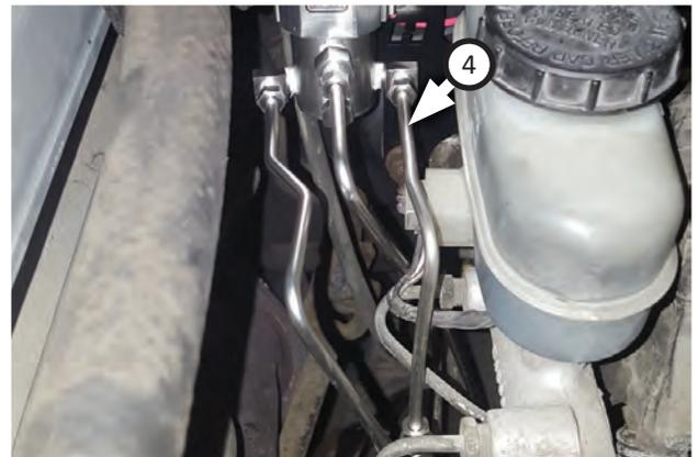
15. Install **brake line (4)**; left front brake line to left side of solenoid and union on factory left side brake line.
