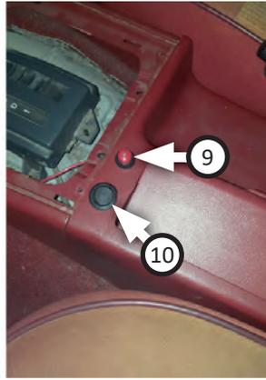
23. Drill and mount **On/Off switch (10)** and **lit momentary switch (9)** to center console as shown.
