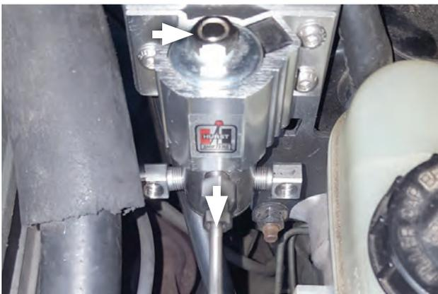
**NOTE:** Solenoid can swivel by loosening nut on top. Only hand tighten lines until they are all installed.
