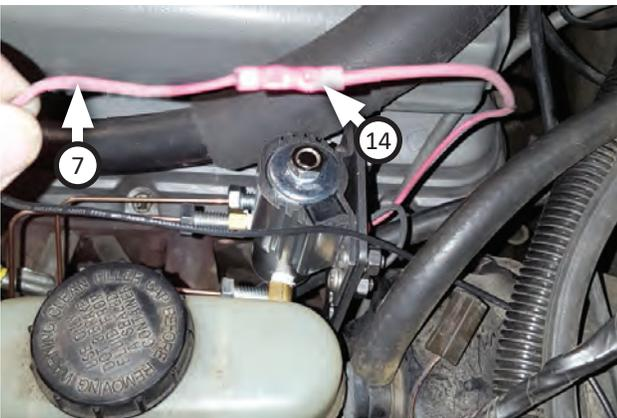
20. Connect red wire (7) to power wire with splice connector (14) and trim just enough red wire to reach from solenoid to vehicle interior.
