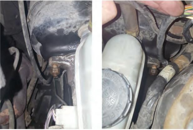
8. Remove (x2) nuts that mount master cylinder to brake booster. Do NOT remove master cylinder.
