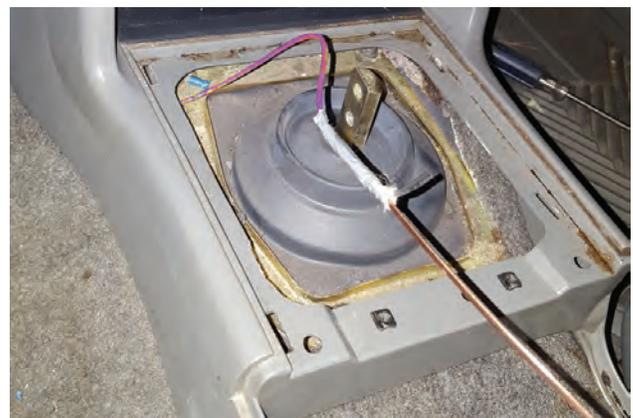
22. To mount switches on center console, pull carpet back then draw power wire through to center console as shown.
