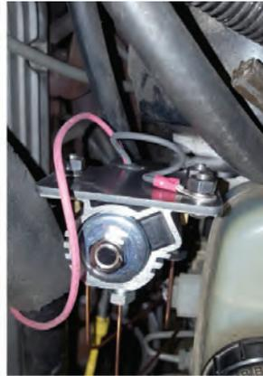
19. Ground solenoid to bracket using eyelet (13).
