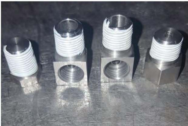
3. Apply teflon tape to all pipe threads.
