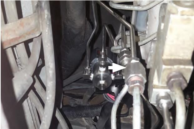
16. Install **brake line (3)**; right front brake line to right side of solenoid and union on factory right side brake line.
