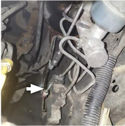
12. Remove right front brake line from proportioning valve. This should be brake line closest to firewall.
