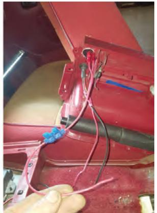
27. Install **terminal (12)** to **red wire (7)** then plug it into on/off switch remaining post. Install **fuse holder (11)**.
