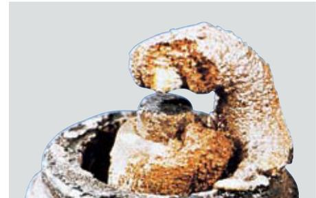
7. Center electrode covered with melted deposits
