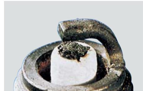
8. Partially melted center electrode
