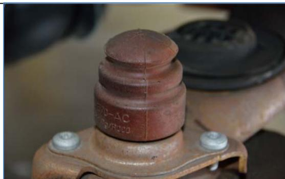
2) Cut out each OE bump stop while holding in a vice as shown. Some prying may be required to get the last bit out.
