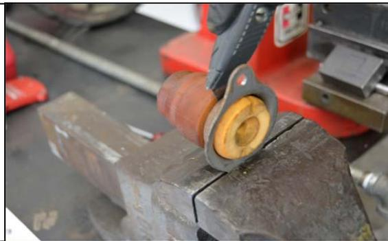
3) Squeeze the new Hurst bump stops into place as shown. A small bit of grease helps.
