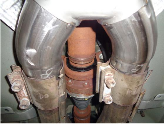
2) Place the factory intermediate pipes with the clamps in place onto the back of the new Flowmaster Scavenger X-pipe and slide the pipes fully together. Center the clamps on the connections and tighten enough to hold in place.
