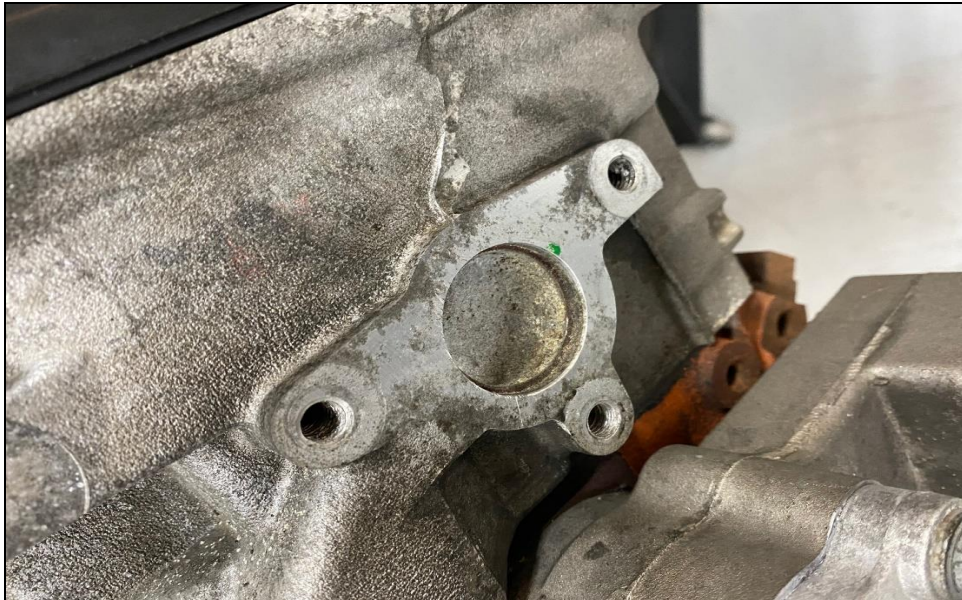
Figure 1 – Gen III Hemi Power Steering Pump Mounting Surface
