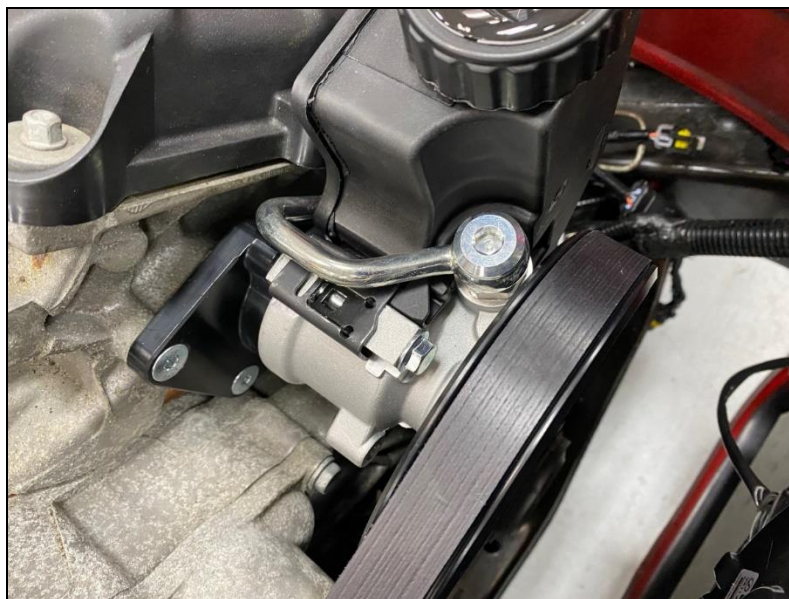
Figure 7 – Hardline Power Steering Pump Installed
