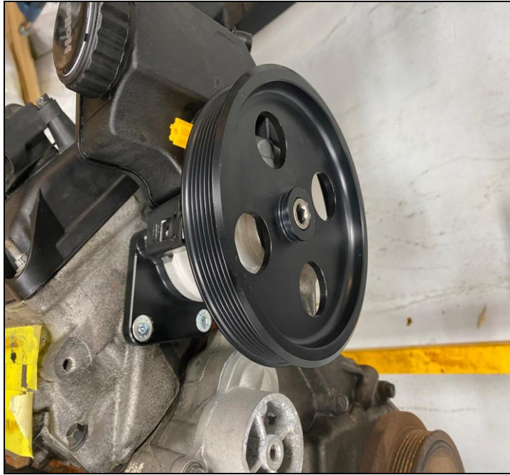
Figure 5 – 198-104/97-383 Assembly Installed onto 97-380 Adapter
