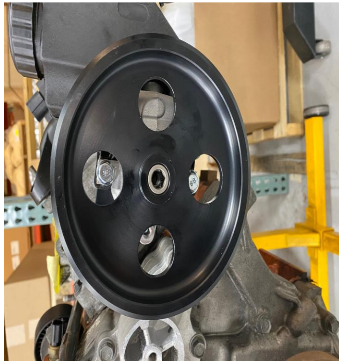
Figure 6 – 197-104 Bolt Access
