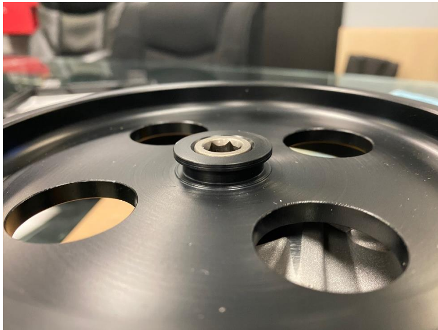
Figure 4 – 97-383 Pulley Installed onto 198-104 Power Steering Pump
