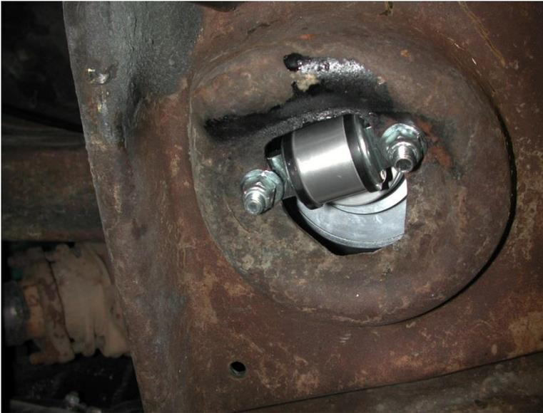
12. Lift the lower control arm up to the CoilOver and tighten with two 3/8" x 1 1/4" bolts, nylocs and flat washers.
