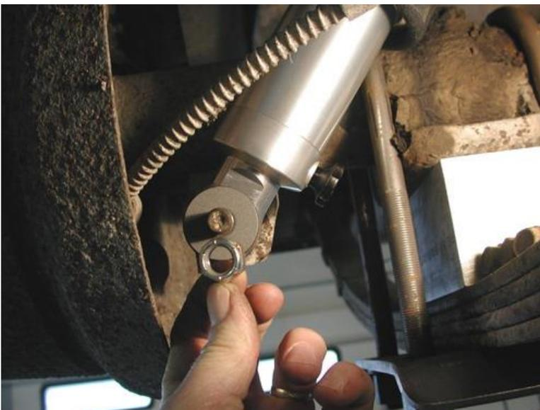
12. Secure the Shockwave to the stud using the  $\frac{1}{8}$ " thick  $\frac{1}{2}$ " inside diameter washer and  $\frac{1}{2}$ " Nylok nut.
