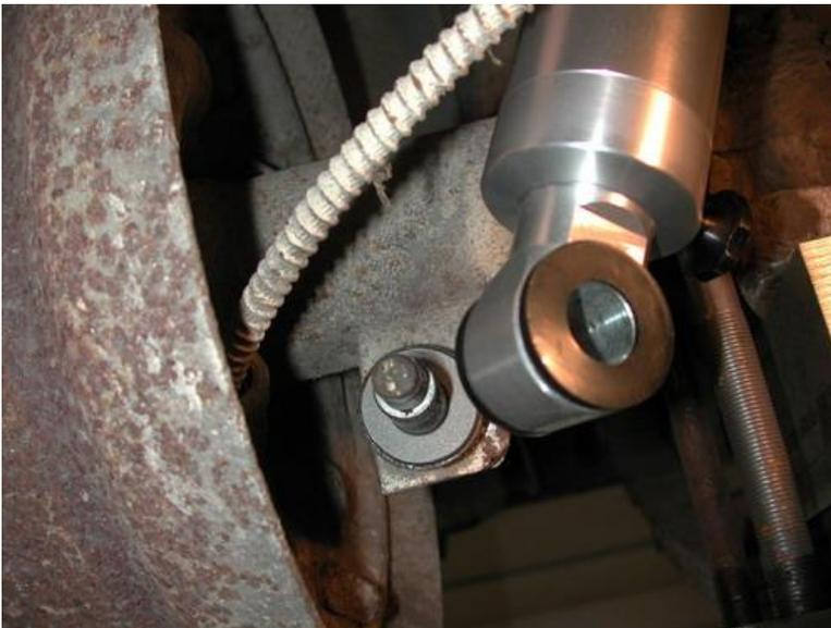
11. Place the  $\frac{1}{8}$ " thick steel washer with the  $\frac{11}{16}$ " inside diameter over the factory lower shock stud on the axle. Then slide the Shockwave over the stud.
