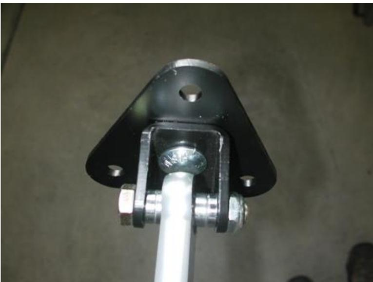
8. The ShockWave must be bolted to the car with the upper mounting bolt running front to rear.
