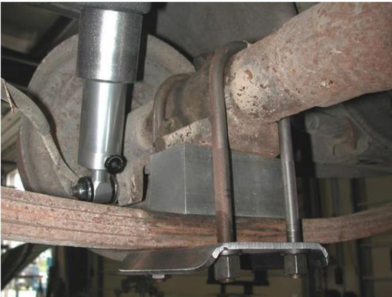
7. Hang the U-bolts over the axle. Position the U-bolt plate under the leaf springs so that the larger hole in the plate aligns with the Allen bolt and nut. Secure the assembly with the four 5/8" nuts and lock washers supplied.
