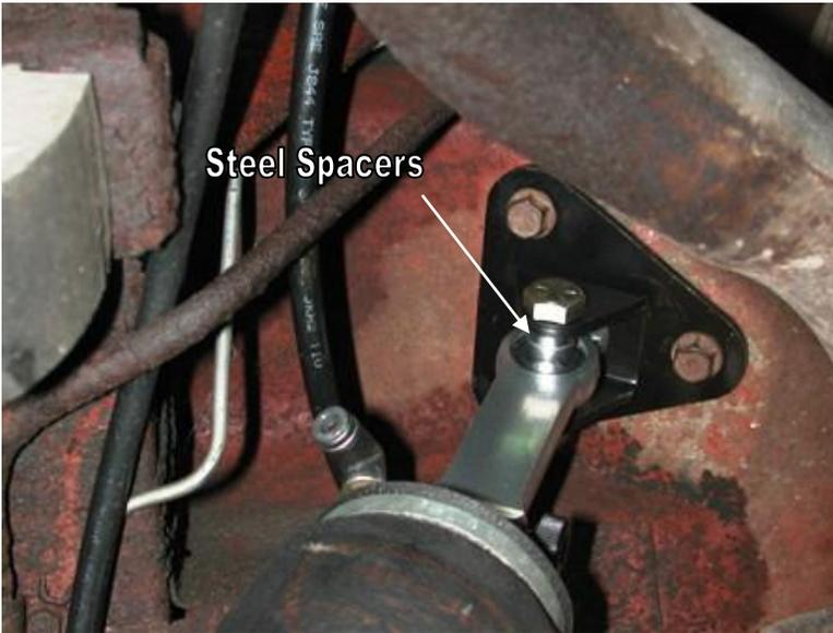
10. Bolt the plate to the factory shock mount holes using the factory bolts.
