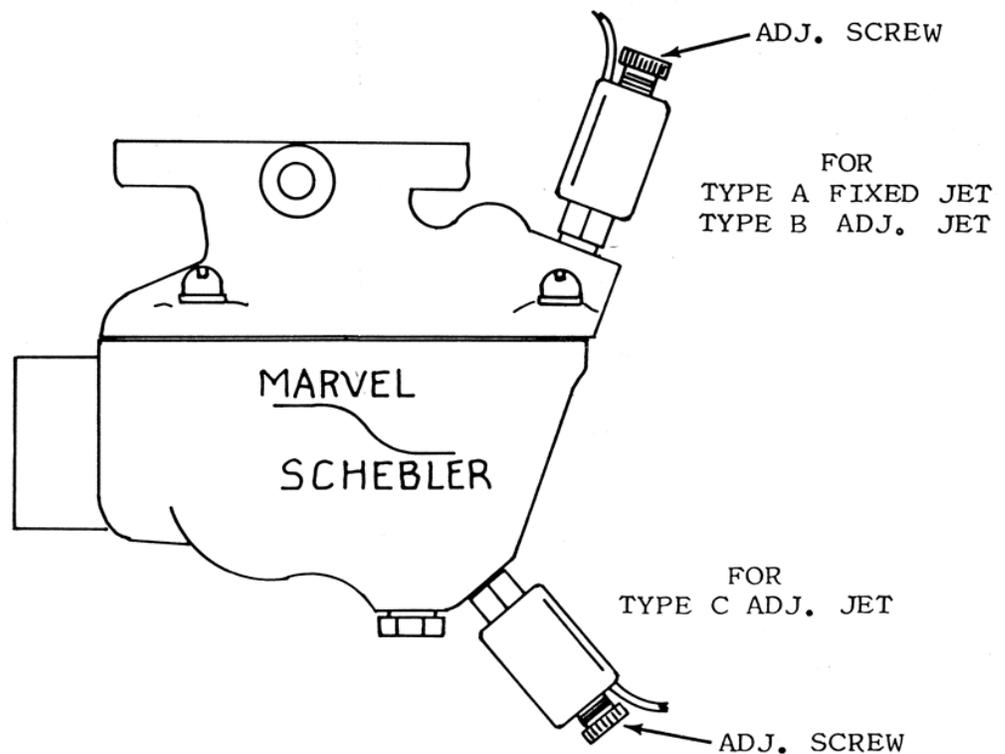
PRELIMINARY SETTING. TURN ADJUSTMENT SCREW IN LIGHTLY UNTIL NEEDLE SEATS, THEN BACK OUT 2-3 TURNS. FINAL SETTING UNDER LOAD IN ACCORDANCE WITH YOUR ENGINE MANUAL.
