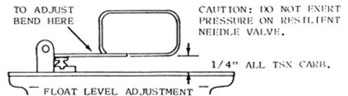
MEASURE FROM GASKET SURFACE TO NEAREST EDGE OF EACH FLOAT. TO ADJUST, BEND FLOAT LEVER KEEPING EDGE OF FLOAT PARALLEL WITH GASKET.
