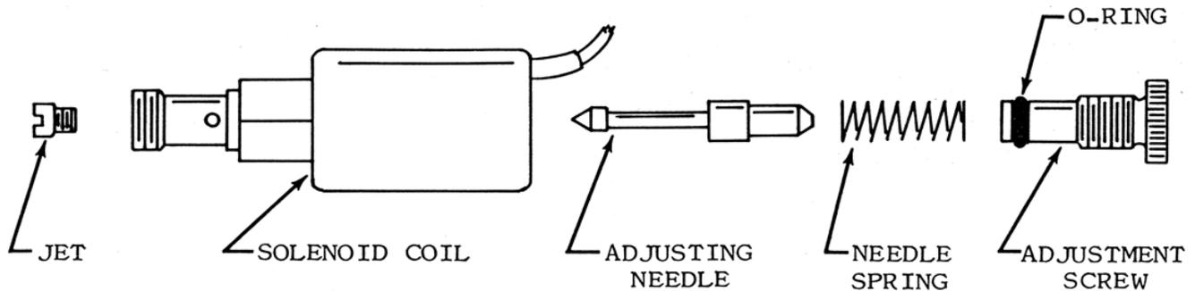
ASSEMBLY: LIGHTLY OIL O-RING AND REASSEMBLE IN REVERSE ORDER OF DISASSEMBLY.
