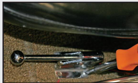
Figure 2A: Securing the trunk release lever.
