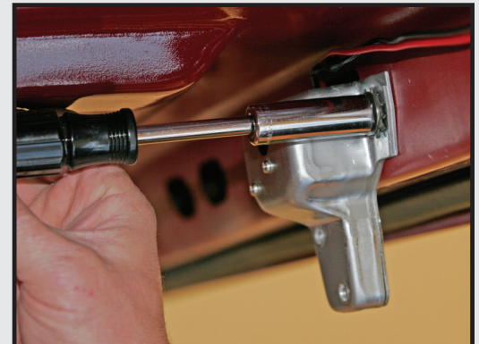
Figure 1A: Mounting the new electric trunk latch on a 1965-66 Mustang.
